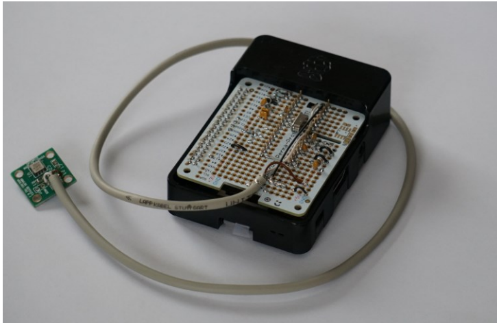
EDGE device Raspberry Pi3 with MEMS sensor
